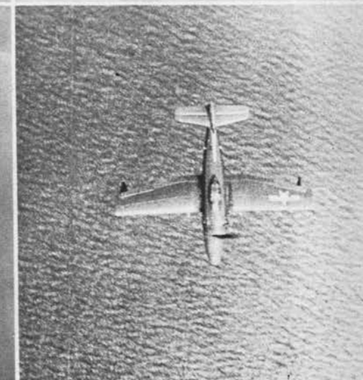
In all views, the Sea Hawk retains its distinctive appearance. Its head-on and overhead resemblance to the F6F is offset by a large single-strut float, tail fairing and cockpit blister.
